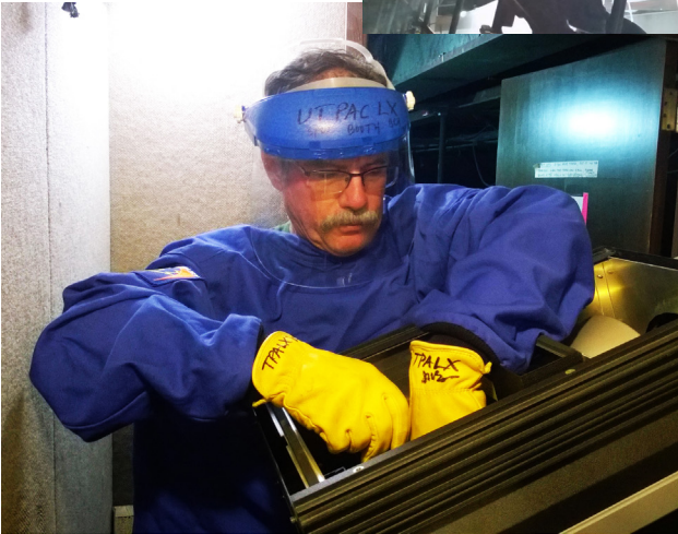
Brother Jeff Ellinger relamping a Lycian 3K at Bass Concert Hall: face shield, gloves, blast coat
